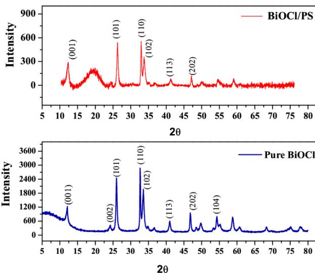
FIGURE 1. X-ray diffraction pattern of as prepared pure BiOCl and BiOCl/PS nanocomposite
