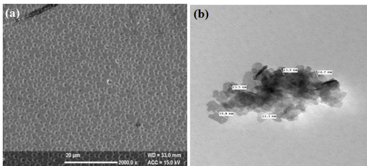
**FIGURE. (a)** SEM image, **(b)**TEM image of BiOCl/PS nanocomposite
