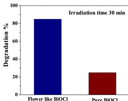
**FIGURE 5.** Photocatalytic activity of flower like BiOCl and Pure BiOCl
