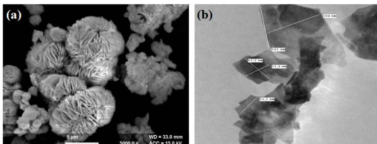
FIGURE 2. (a) SEM image, (b) TEM image of as prepared BiOCl
