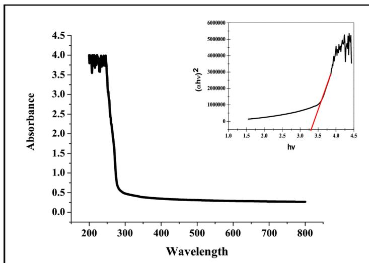
**FIGURE 4.** UV-Vis spectrum of BiOCl/PS nanocomposite
