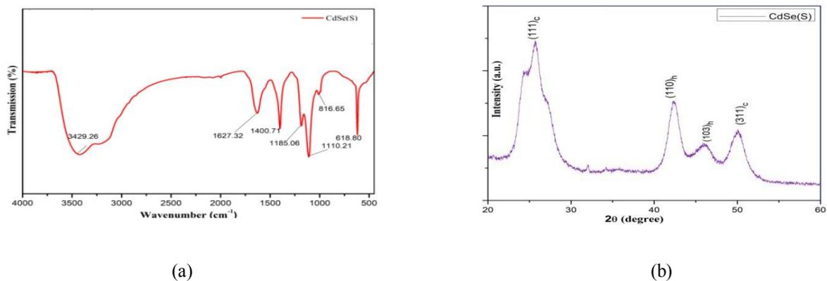
FIGURE 1. (a) FTIR and (b) XRD spectra of CdSe QDs.
