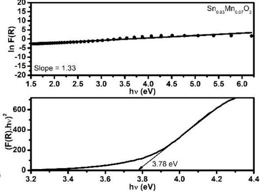
Figure-4: Urbach and Tauc plot for Sn<sub>0.93</sub>Mn<sub>0.07</sub>O<sub>2</sub>
