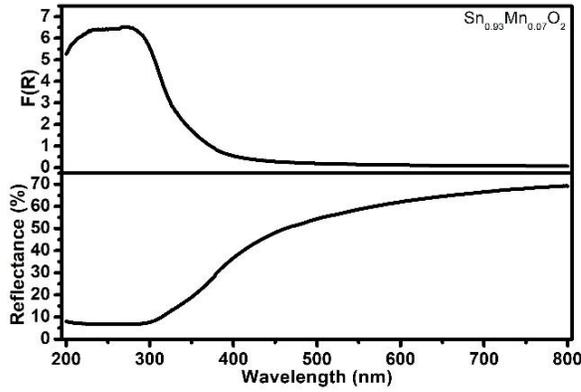
Figure-3: Reflectance and absorbance spectra of Sn<sub>0.93</sub>Mn<sub>0.07</sub>O<sub>2</sub>
