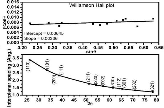
Figure-2: Interplanar spacing and Williamson Hall plot for  $\text{Sn}_{0.93}\text{Mn}_{0.07}\text{O}_2$
