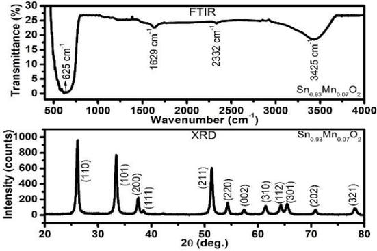
Figure-1: XRD and FTIR spectra of  $\text{Sn}_{0.93}\text{Mn}_{0.07}\text{O}_2$
