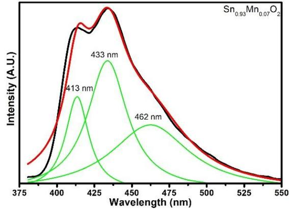
Figure-5 Deconvolution of the emissionspectrum of  $\text{Sn}_{0.93}\text{Mn}_{0.07}\text{O}_2$
