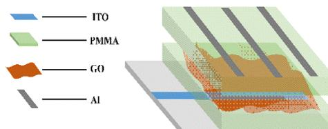
FIGURE 1. Schematic diagram of ITO/PMMA/GOs/PMMA/Al device
