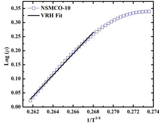
FIGURE 2. Fitted data of Resistivity using VRH model
