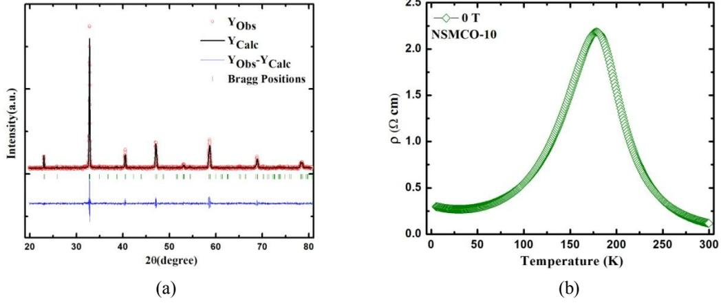
**FIGURE 1.** (a) XRD with Rietveld Refinement, (b) Resistivity as a function of Temperature at 0 T.
