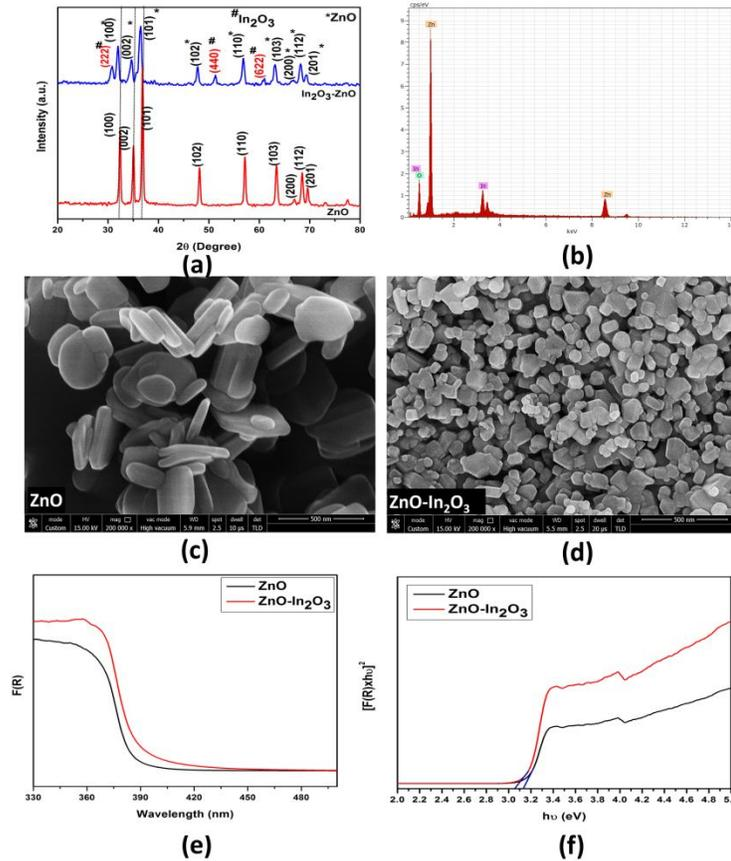
**FIGURE 1.** XRD spectra (a) EDS image (b) FESEM micrographs of pristine ZnO and ZnO-In<sub>2</sub>O<sub>3</sub> (c,d) UV-Vis spectra (e) and Tauc's plot (f) of the samples.
