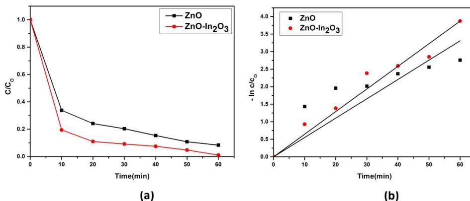
FIGURE 2. MB degradation spectra (a) and rate constant calculation spectra (b) of the samples.
