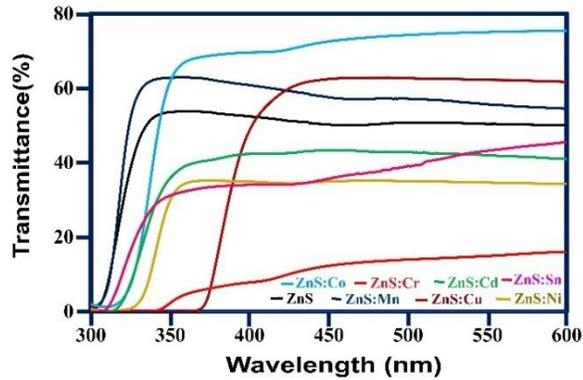
FIGURE 3.a)UV-Transmittance peaks of ZnS with different elements
