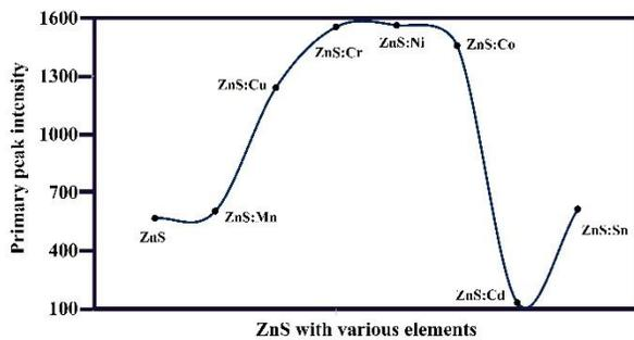
FIGURE 1. b) Peak intensity vs doped elements with ZnS QDs.
