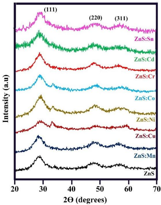
FIGURE 1.a) XRD patterns of ZnS with different elements
