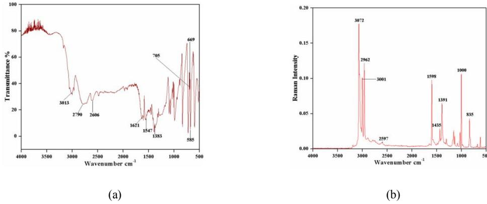
FIGURE 2. (a) FTIR spectrum of PBA crystal, (b) FT Raman spectrum of PBA crystal.
