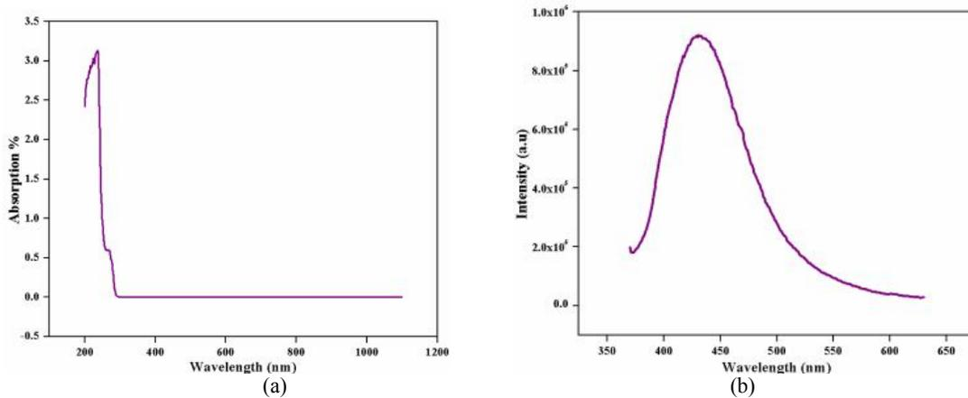
FIGURE 3. (a) UV visible spectrum of PBA crystal, (b) Fluorescence spectrum of PBA crystal
