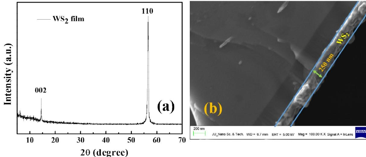
FIGURE 1. (a) XRD pattern of WS<sub>2</sub> thin film (b) Cross-sectional FESEM image of the grown film.
