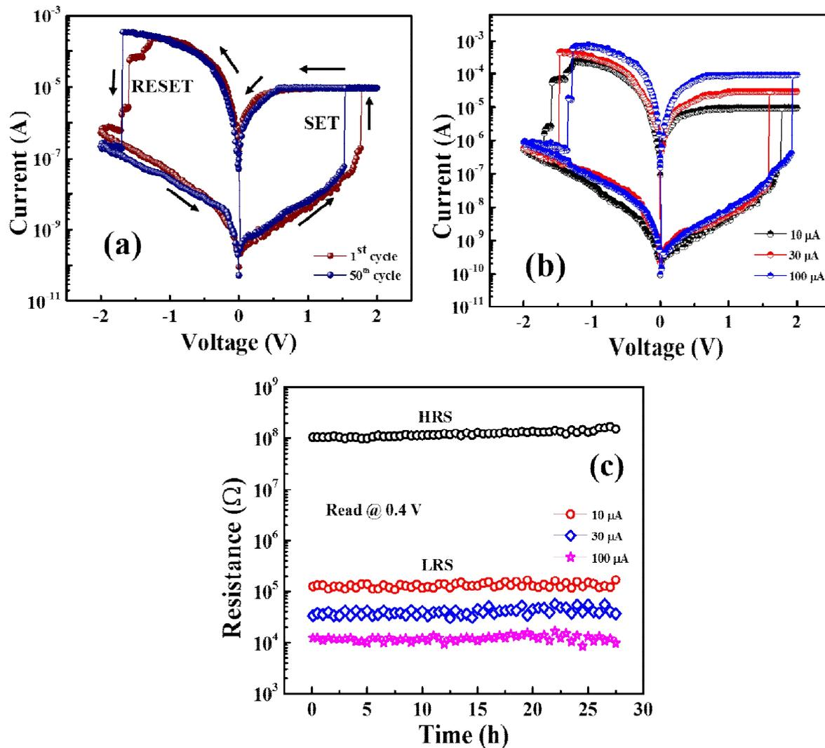
**FIGURE 2.** (a) Bipolar current versus voltage graph of the Al/WS<sub>2</sub>/Pt memory device (b) Multilevel conductance curve for various compliance current (c) retention characteristic of different resistance states under a constant read voltage (0.4 V).
