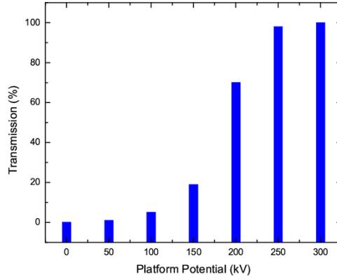
**FIGURE 5.** Transmission of beam intensity with platform potential.
