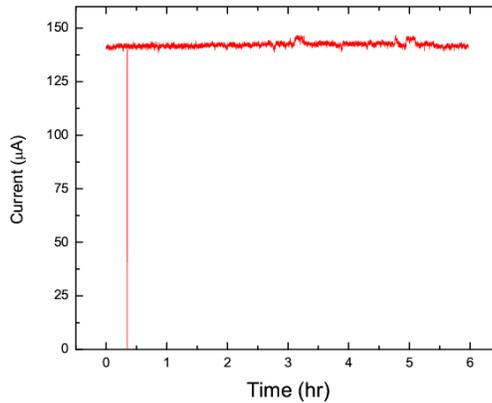
**FIGURE 2.** Stability test for Ar<sup>8+</sup> ions up to 6 hrs.
