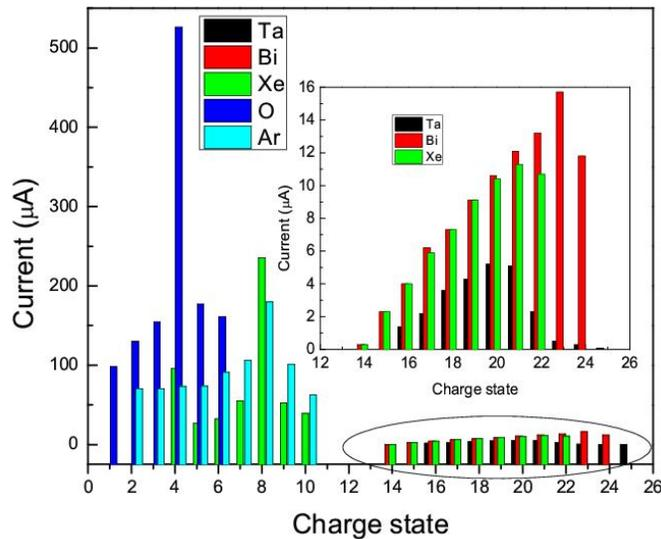
**FIGURE 4.** Beam intensity distribution with change states for different ions
