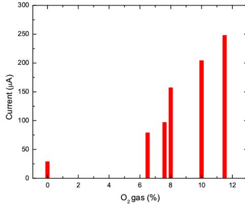
**FIGURE 3.** Effect of support gas (O<sub>2</sub>) on the intensity of the current of Ar ions. The current increases with increase in the quantity of the support gas.
