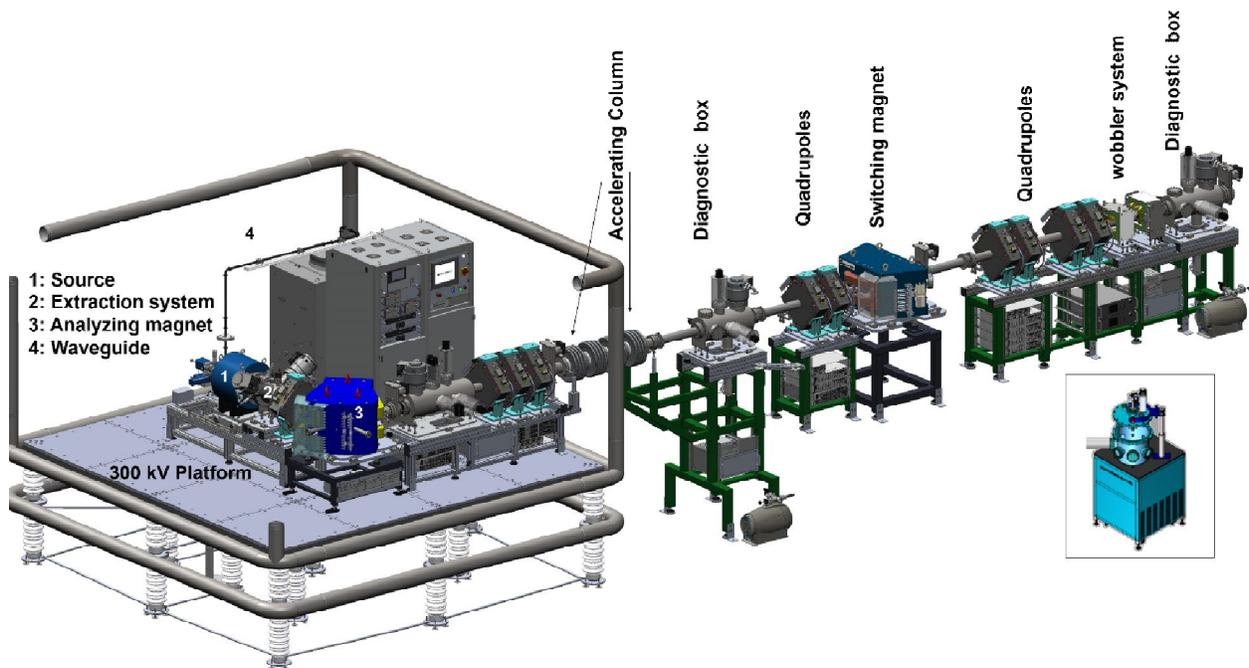
**FIGURE 1.** 3D view of the Supernanogan ECR with zero degree beam line installed at University of Allahabad. Experimental chamber is shown in inset in the figure.
