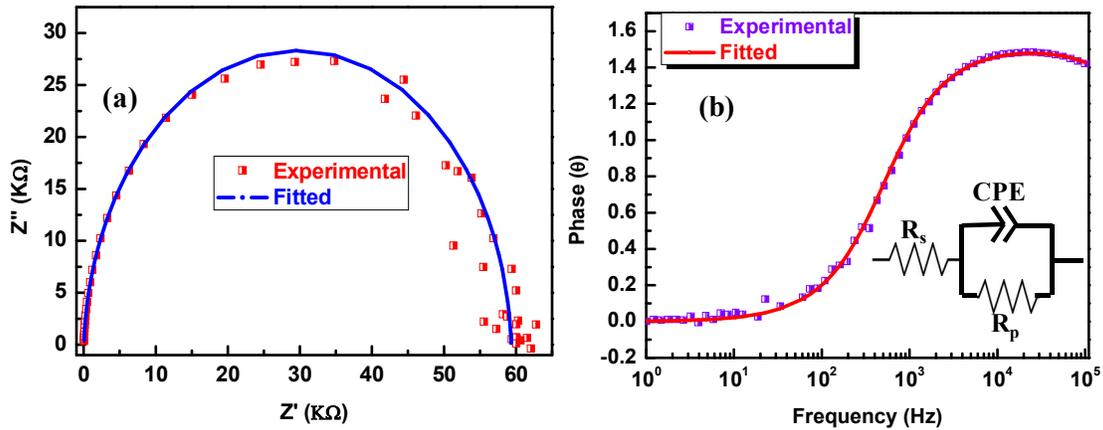
**FIGURE 3.** Impedance analysis of the solar cell device (a) Nyquist plots of PTB7:PC<sub>70</sub>BM based device (b) Bode plot of PTB7:PC<sub>70</sub>BM based device, inset figure of (b) shows electrical equivalent circuit that was used in simulation and curve fitting.
