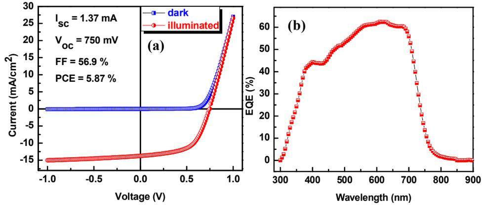
**FIGURE 2(a).** J-V curve under dark and illumination of ITO/ZnO/PTB7:PC<sub>70</sub>BM/MoO<sub>3</sub>/Ag device, **(b)** External Quantum Efficiency curve of the device.
