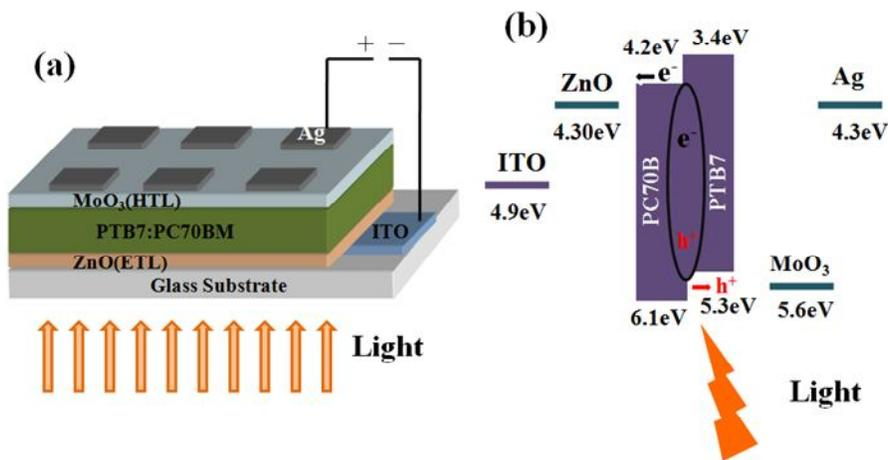
**FIGURE 1.** Schematic for an inverted organic solar cell structure and its corresponding energy level diagram.
