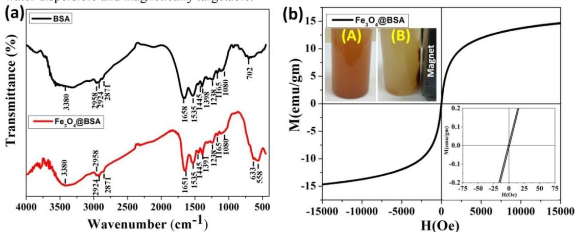
**FIGURE 3.** (a) FTIR patterns of pure BSA and  $Fe_3O_4@BSA$  nanocarrier. (b) Room temperature M-H curve of  $Fe_3O_4@BSA$  nanocarrier. Inset at the top of fig. (b) shows aqueous dispersion of  $Fe_3O_4@BSA$  nanocarrier, (A) without magnet and (B) with magnet. Inset at the bottom of fig. (b) shows enlarged M-H curve of  $Fe_3O_4@BSA$  nanocarrier.
