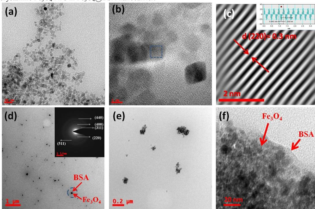
**FIGURE 2.** (a) TEM and (b) HRTEM micrographs of  $\text{Fe}_3\text{O}_4$  NPs. (c) IFFT image for selected region (blue color) of fig 2(b). Line profile through atomic planes is shown in inset of fig (c). (d-f) TEM micrographs of  $\text{Fe}_3\text{O}_4@$ BSA nanocarrier at different magnifications. Indexed SAED pattern of  $\text{Fe}_3\text{O}_4@$ BSA nanocarrier is shown in inset of figure 2 (d).
