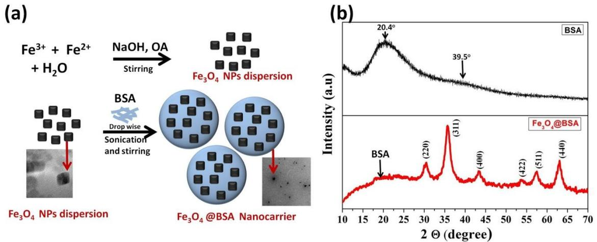
**FIGURE 1.** (a) Schematic diagram showing formation mechanism of  $\text{Fe}_3\text{O}_4$  NPs and  $\text{Fe}_3\text{O}_4@$ BSA nanocarriers. (b) XRD patterns of pure BSA powder and  $\text{Fe}_3\text{O}_4@$ BSA nanocarrier.
