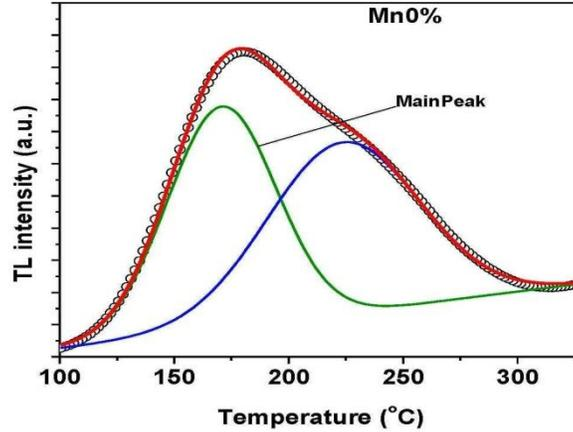
FIGURE 2. TL de convoluted glow curve of  $\text{CaYAl}_3\text{O}_7: \text{Mn}^{2+}$  (0.0 mol %) with 100Gy.
