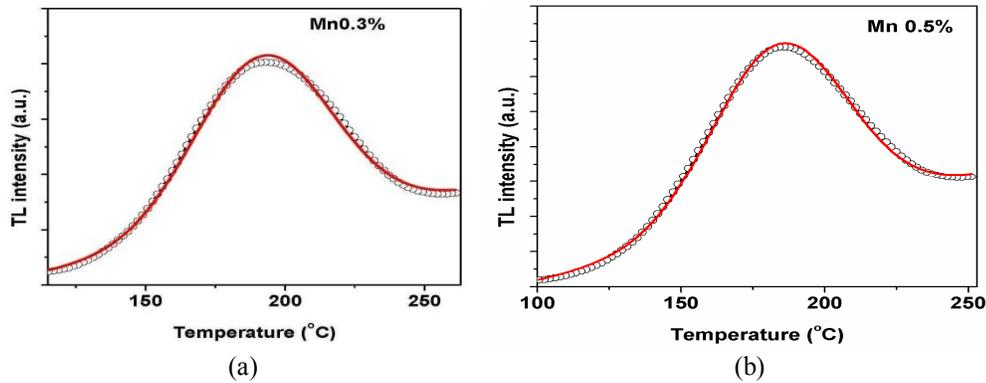
FIGURE 3. TL de convoluted glow curve of (a)  $\text{CaYAl}_3\text{O}_7: \text{Mn}^{2+}$  (0.3 mol %) and (b)  $\text{CaYAl}_3\text{O}_7: \text{Mn}^{2+}$  (0.5 mol %) with fixed 100 Gy gamma dose.
