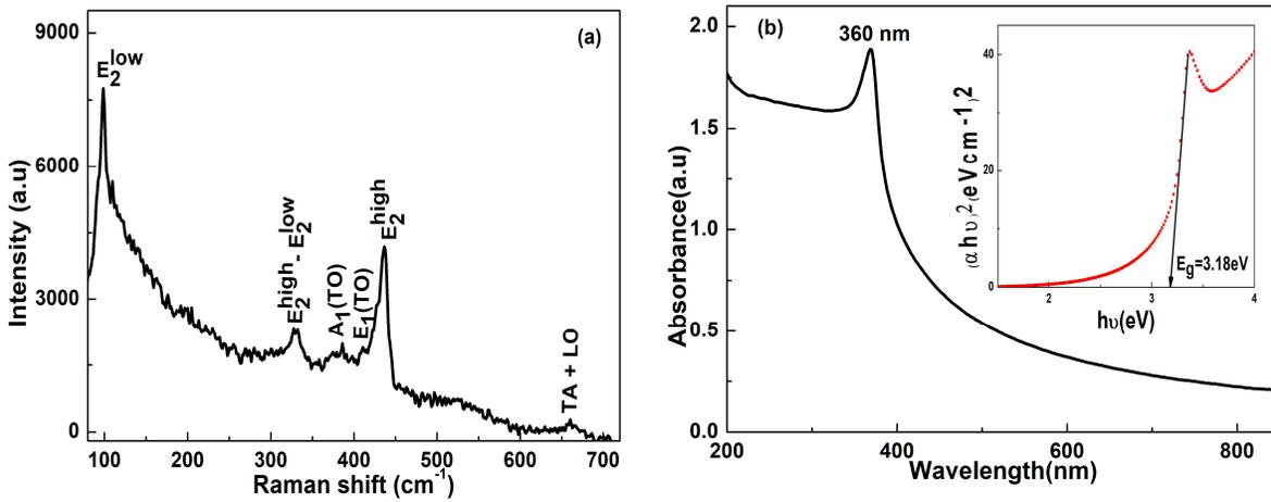
FIGURE 2.(a)Raman spectra, (b) UV-vis absorption spectra with inset Tauc plot for synthesized ZnO nanoparticles.
