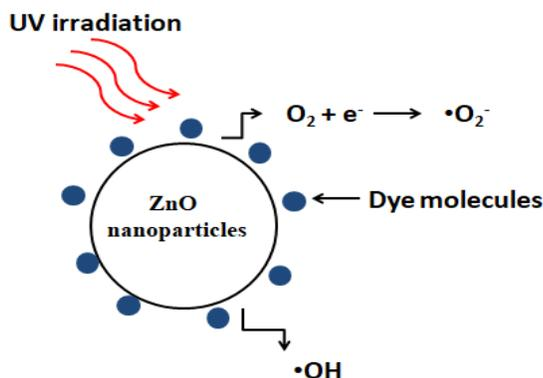
**FIGURE 4.** Schematic of mechanism involved in photodegradation of dye by ZnO nanoparticles.
