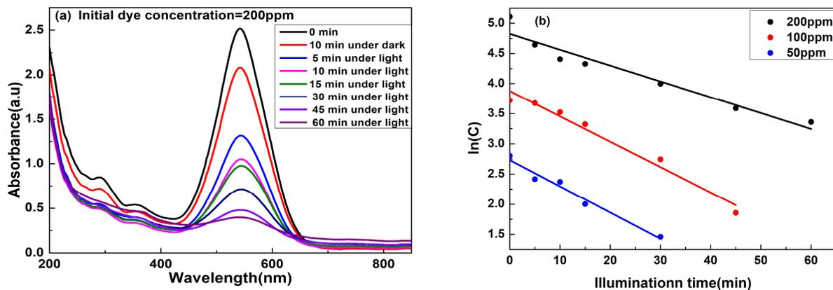
**FIGURE 3.**(a)UV-Visible spectra of treated direct violet dye of 200 ppm initial concentration,(b)pseudo first order kinetics of dye with initial concentration equal to 200,100 and 50 ppm.
