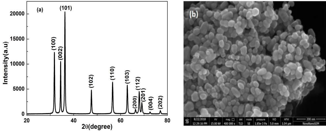
FIGURE 1.(a)XRD pattern, (b)SEM image of synthesized ZnO nanoparticles.
