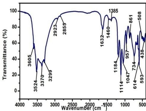
**FIGURE 2.** FT-IR spectra of ZnO NPs.
