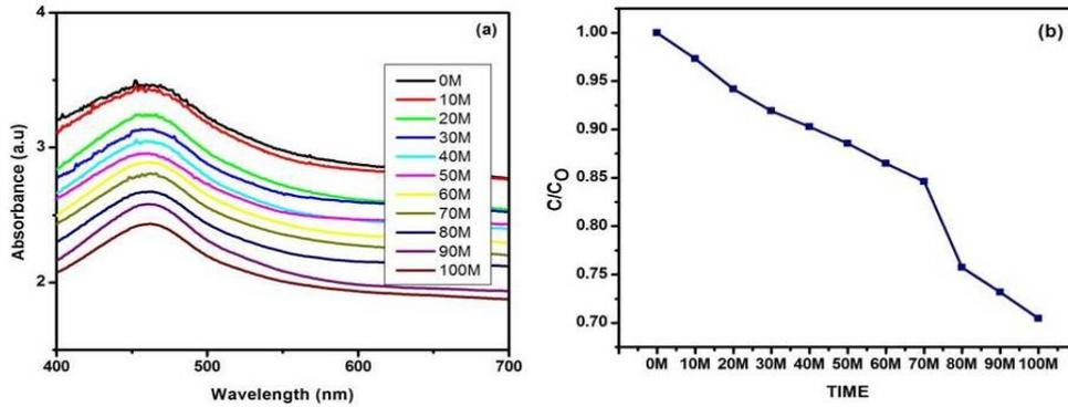
FIGURE 4. (a) Photo degradation of dye by ZnO NPs (b) Photo catalytic activity of ZnO NPs under UV light, plotted as a function of time.
