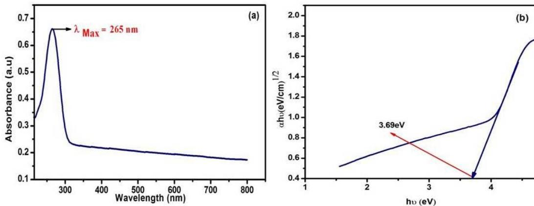
FIGURE 1. (a) UV-Vis spectrum of ZnO NPs and (b) Tauc's plot of ZnO NPs.
