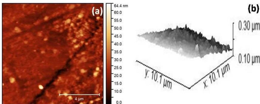
**FIGURE 3.** (a) 2-D morphological structure of ZnO NPs (b) 3-D morphological structure of ZnO NPs
