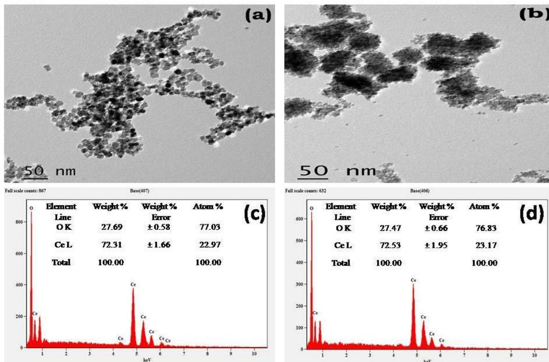
FIGURE 2. (a) TEM image of HYNP (b) TEM image of CONP (c) EDS graph of HYNP (d) EDS graph of CONP.
