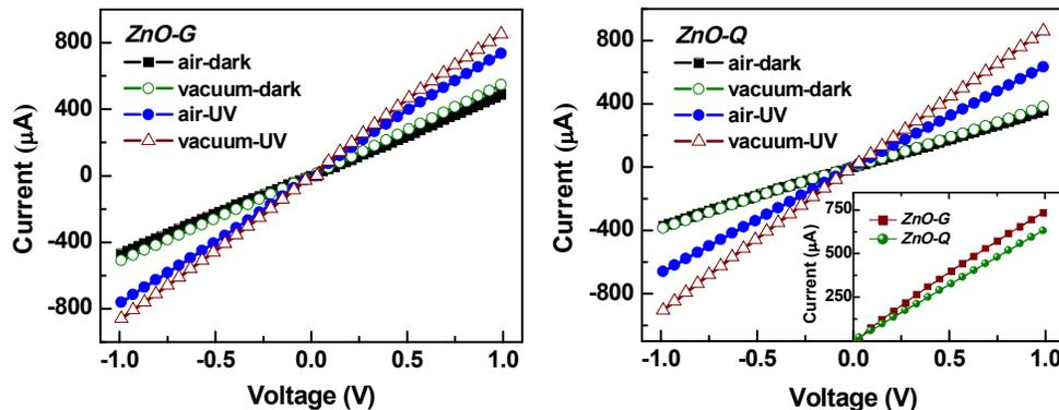
FIGURE 2. Current versus voltage plots of *ZnO-G* and *ZnO-Q* samples. The inset figure shows comparison of photocurrent for both samples in air.
