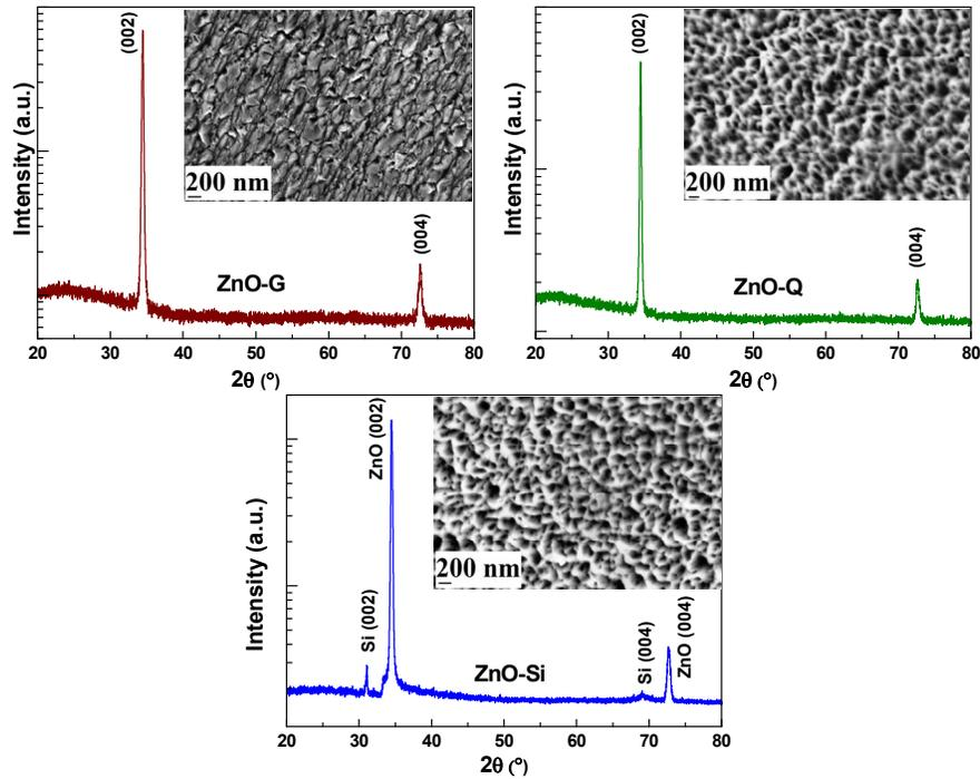
**FIGURE 1.** XRD patterns and respective SEM images of ZnO nanostructured thin films grown on glass, quartz and Si (001) substrates.
