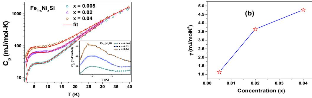
**FIGURE 1.**(a) Log plot heatcapacity (HC)vs temperature of  $\text{Fe}_{1-x}\text{Ni}_x\text{Si}$  ( $x = 0.005, 0.02, 0.04$ ) at zero field of low temperatures below 40 K. Inset: HC at low temperature below 10 K of  $\text{Fe}_{1-x}\text{Ni}_x\text{Si}$ . (b) Sommerfeld coefficient ( $\gamma$ ) of  $\text{Fe}_{1-x}\text{Ni}_x\text{Si}$  vs concentration.
