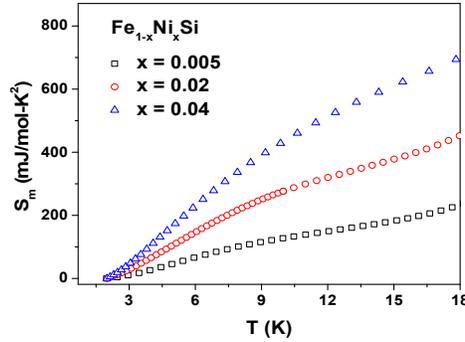
**FIGURE 2.** Magnetic entropy of Fe<sub>1-x</sub>Ni<sub>x</sub>Si (x = 0.005, 0.02, 0.04) at low temperatures.
