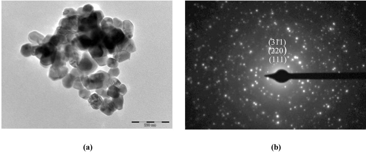
**FIGURE 2.** (a) Confirm the formation of  $\text{Co}_3\text{O}_4$  nano particles. (b) The Selected area diffraction pattern of nano particles confirms the phase formation.
