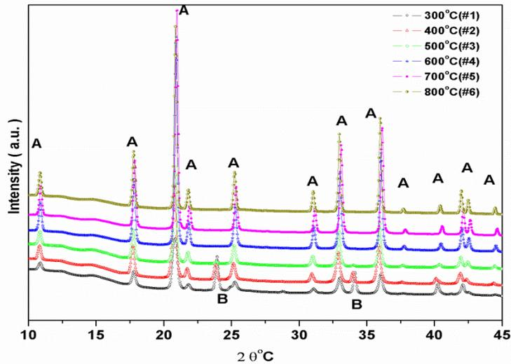
**FIGURE 1.** X-Ray Diffraction patterns for samples (#1 to #6) of cobalt oxide annealed in air at various temperatures. Samples (#1 to #3) show mixed phase whereas (#4 to #6) show single phase. CoO and Co<sub>3</sub>O<sub>4</sub> phases are represented by symbol B and A, respectively.
