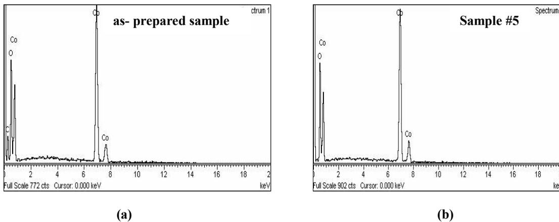
**FIGURE 3.** (a): K-edge EDAX spectra of as-prepared sample (b) sample #5 (annealed at  $700^\circ\text{C}$ )
