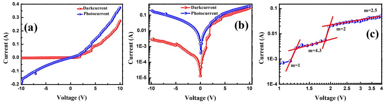
**FIGURE 2:** FTO/TiO<sub>2</sub>/CH<sub>3</sub>NH<sub>3</sub>PbBr<sub>3</sub>/PEDOT:PSS/Al (a) I-V characteristics of the perovskite device in dark & light, (b) I-V characteristic in semi logarithmic scale of device, (c) double-logarithmic plot of the device.
