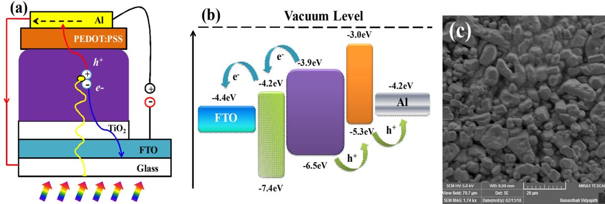
**FIGURE 1.** (a) Energy level sketch of materials used in the fabrication of device, (b) schematic device structure of the perovskite based device, (c) FESEM image of CH<sub>3</sub>NH<sub>3</sub>PbBr<sub>3</sub> perovskites film.
