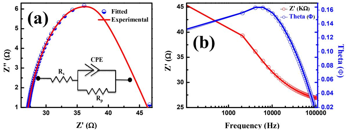
**FIGURE 3.** (a) Nyquist plot of the device under study, inset shows electrical equivalent circuit of the device, (b) Bode plots of the device in dark condition.
