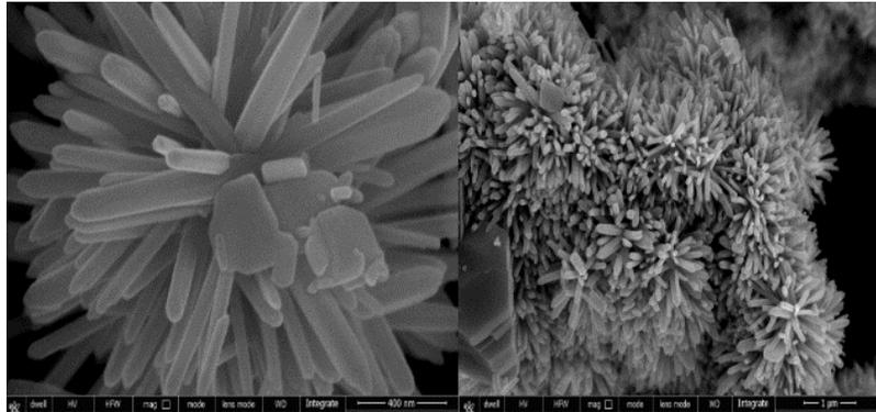
**FIGURE 2.** FESEM micrographs of as-synthesized ZnO-400
