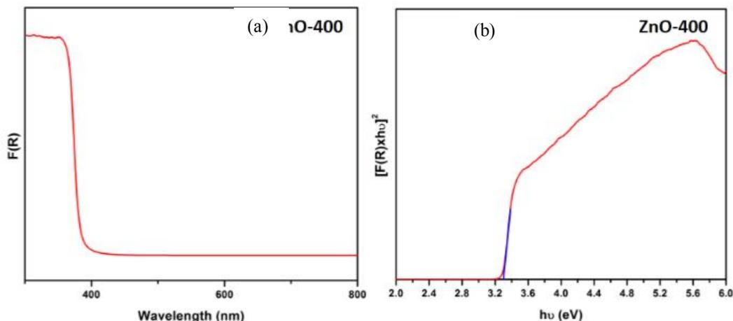
FIGURE 3. Diffuse reflectance spectra (a) and Taucs plot (b) of ZnO-400.
