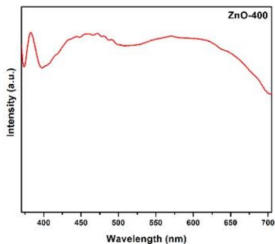
FIGURE 4. Photoluminescence spectra of ZnO-400.
