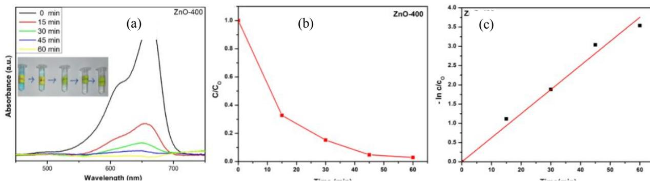
**FIGURE 5.** UV-vis absorption spectra of MB at different time in the presence of ZnO-400 (a) MB degradation spectra (b) and rate constant calculation spectra (c) of the sample.
