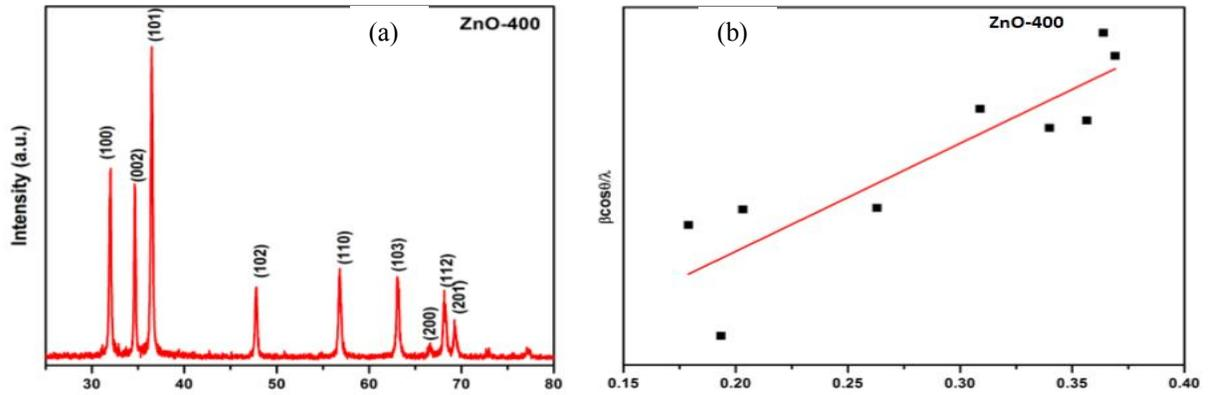
**FIGURE 1.** XRD spectra (a) and W-H plot (b) of ZnO-400.
