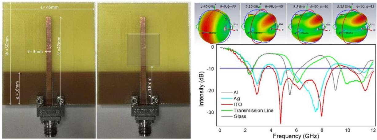
Figure 1(a): Model and dimensions of the DRA with transmission line, ground plane and the ITO glass slide arrangement;(b) Above: Simulated Far Field patterns of the ITO antenna at four important Wi-Fi frequencies: 2.45, 5.15, 5.5 and 5.85 GHz; (b) Below:  $S_{1,1}$  parameters of the ITO/glass DRA as compared to Al and Ag metal coated glass slides of same dimensions. A reference response of the bare transmission line and uncoated glass is also shown.
