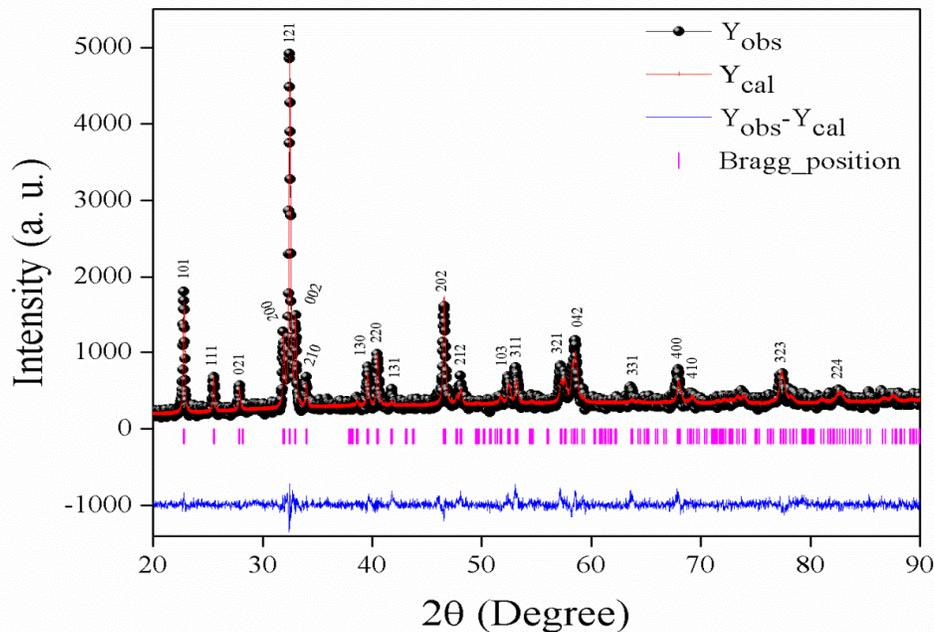
FIGURE 1. Rietveld refined profile of Bi<sub>0.7</sub>Sm<sub>0.3</sub>FeO<sub>3</sub>
