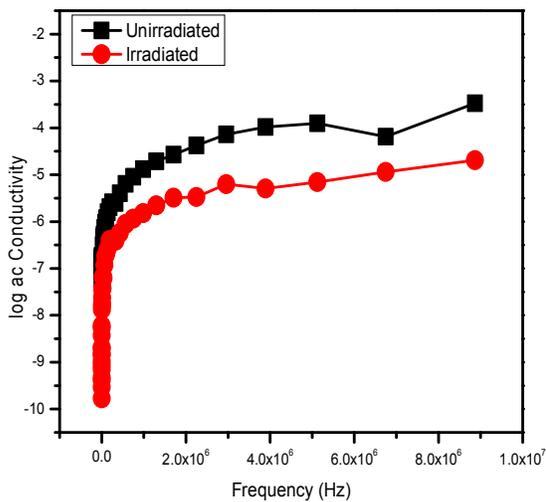
FIGURE 3. Plot of ac conductivity of  $\gamma$ -irradiated PMMA as function of frequency.
