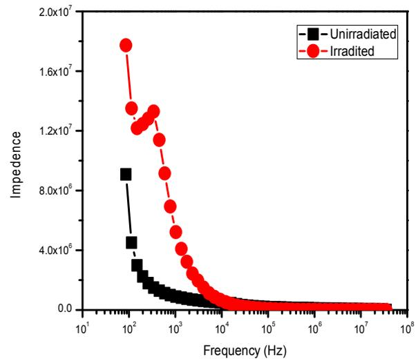
FIGURE 4. Plots of Impedence of gamma irradiated PMMA as function of frequency.
