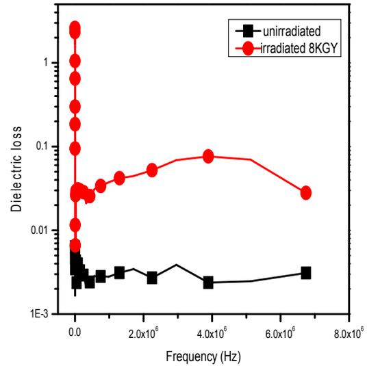
FIGURE 2. Plot of dielectric loss of  $\gamma$ -irradiated PMMA as function of frequency.
