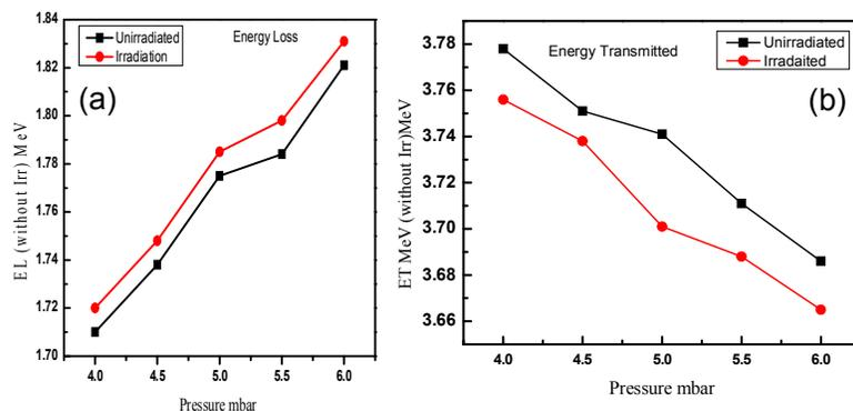
FIGURE 5. Plots of (a) Energy loss, (b) Transmitted energy of Alpha particles in PMMA film.
