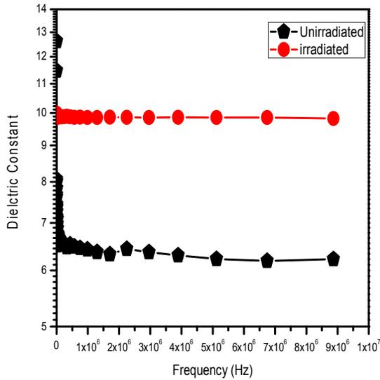
FIGURE 1. Plot of dielectric constant of  $\gamma$ -irradiated PMMA as function of frequency.
