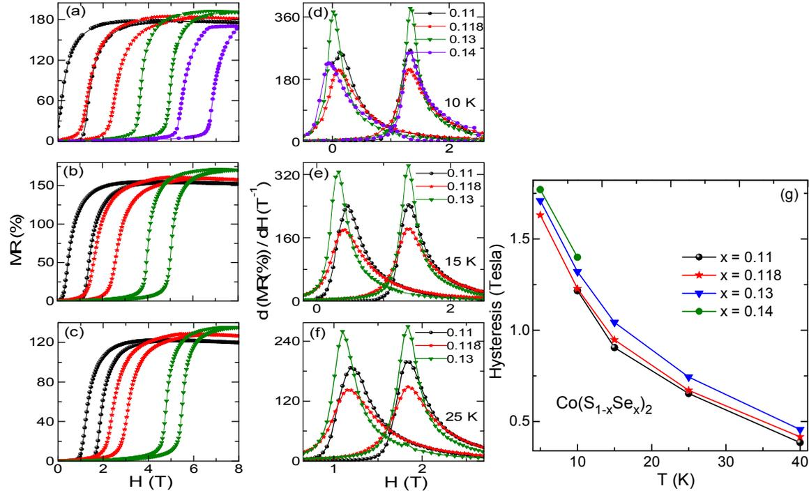
**FIGURE 2** Isothermal MR (left panel) measured at [a] 10 K, [b] 15 K and [c] 25 K for  $\text{Co}(\text{S}_{1-x}\text{Se}_x)_2$ ,  $x = 0.11, 0.118, 0.13, 0.14$  and its derivative are shifted horizontally to match peak position of field increasing cycle with that of  $x=0.11$  as shown in (d)-(f). [g] Shows temperature dependence of hysteresis estimated from above MR measurement.
