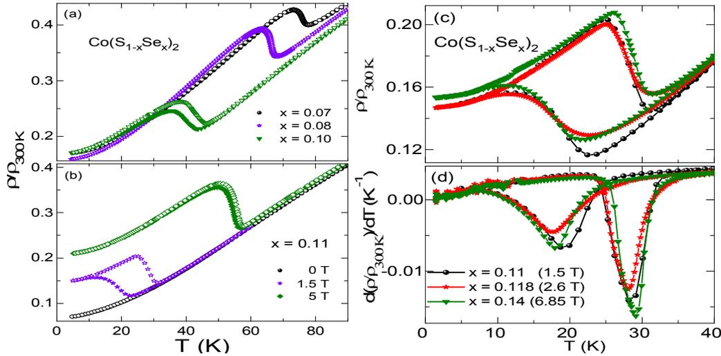
**FIGURE 1**(a)-(b)Temperature dependence of normalized resistivity ( $\rho/\rho_{300K}$ ) for [a]  $x = 0.07, 0.08, 0.1$  in the absence of applied magnetic field and [b]  $x = 0.11$  in the presence of labeled magnetic field.(c)Shows temperature dependence of normalized resistivity ( $\rho/\rho_{300K}$ ) and (d) its derivative for  $\text{Co}(\text{S}_{1-x}\text{Se}_x)_2$  for the labeled  $x$  and  $H$ . ( $x, H$ ) combinations are chosen so that transition temperature becomes nearly equal.
