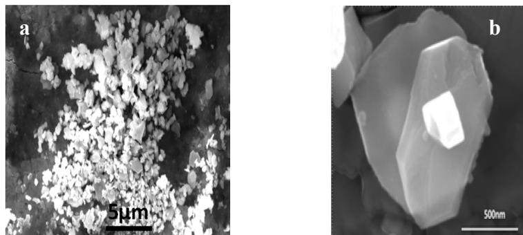
**Figure 2.** FESEM images of nanocrystalline SnSe:(a) Lower magnification and (b) higher magnification
