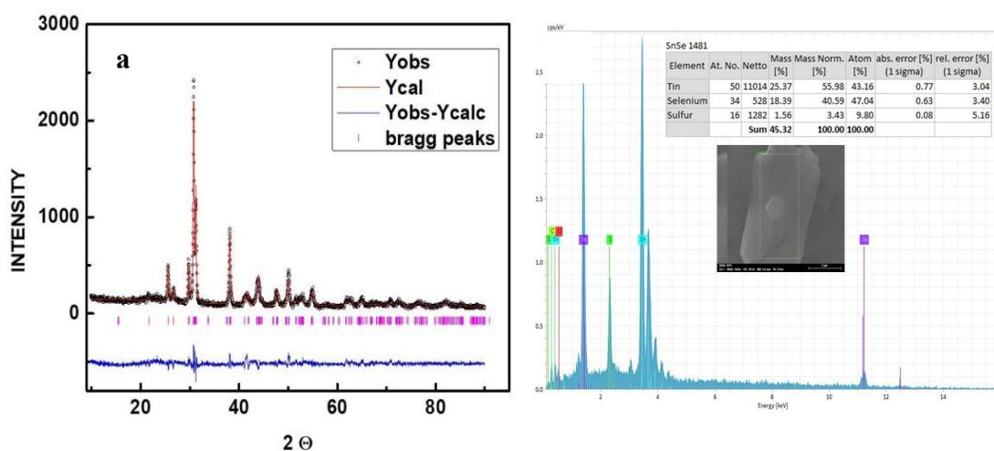
FIGURE 1. (a) Rietveld Refinement of SnSe nanoflakes (b) EDS spectrum (Inset) EDS composition of single SnSe.
