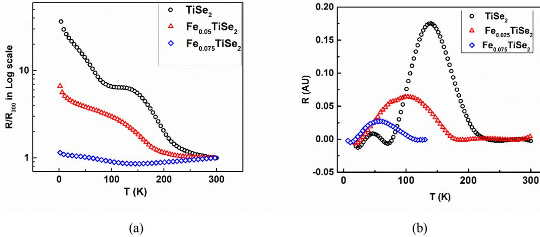
**FIGURE 2.** (a) Resistance vs temperature plot of resistance of  $\text{TiSe}_2$  and its Iron intercalated samples. (b) CDW peaks extracted after background subtraction with proper scaling (curve of  $\text{Fe}_{0.025}\text{TiSe}_2$  multiplied by 10 & curve of  $\text{Fe}_{0.075}\text{TiSe}_2$  multiplied by 100) showing decrease in peak intensity with increasing iron intercalation in  $\text{TiSe}_2$ .
