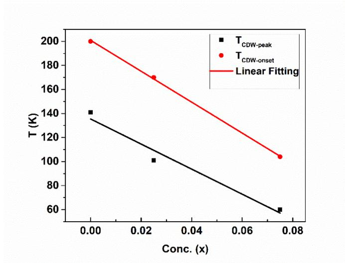
**FIGURE 3.** Linear fitting of Peak temperatures and CDW transition temperatures ( $T_{\text{CDW-onset}}$  &  $T_{\text{CDW-peak}}$ ) that shows a decrease with increase in Fe concentration.
