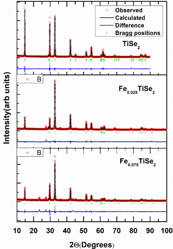
**FIGURE 1.** Rietveld refinement of XRD pattern of  $\text{TiSe}_2$  and its Fe intercalated samples
