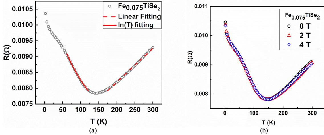
**FIGURE 4.** (a) Semiconductor to metal transition as observed in  $-\ln T$  fitting (solid line) at low temperatures while a linear fitting (dash line) is clear at high temperature. (b) Magnetoresistance transport data showing no effect in resistance.
