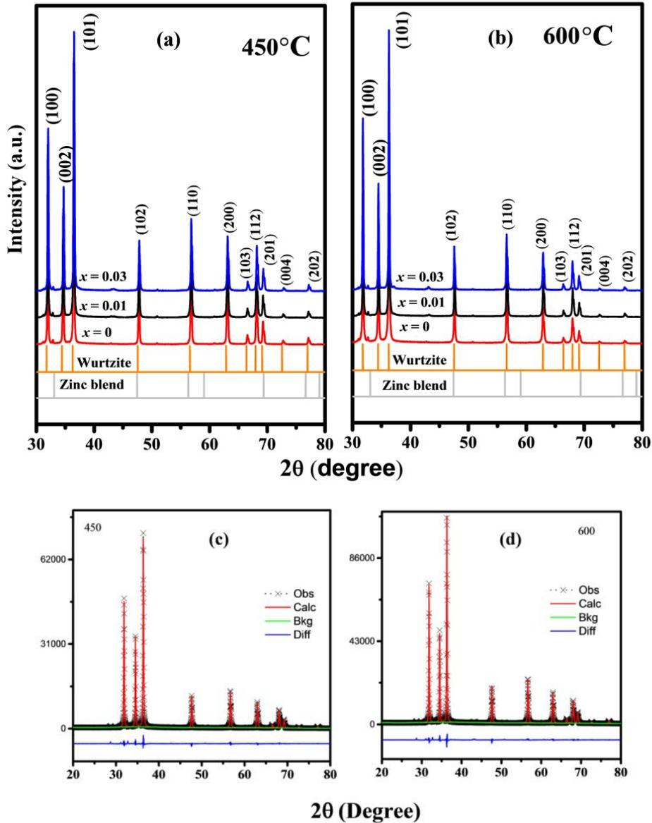
**Figure 1:** (a), (b) XRD pattern of ZnO and Ni doped ZnO for  $x = 0.01, 0.03$  annealed at 450°C & 600°C
