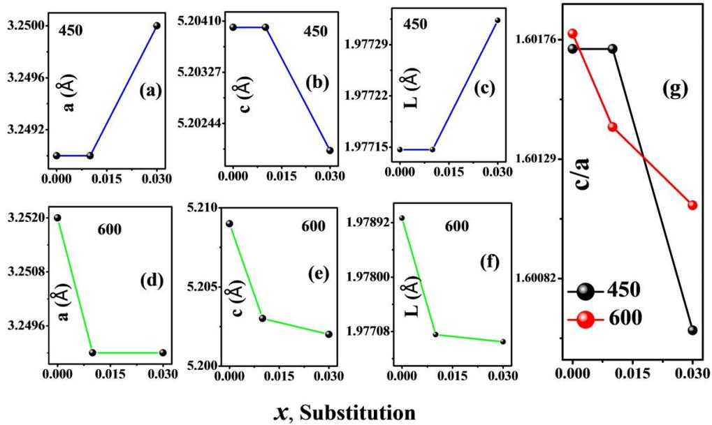
**Figure 2:** (a), (b), (d) and (e) obtained Lattice parameters a and c using GSAS software at 450°C & 600°C respectively
