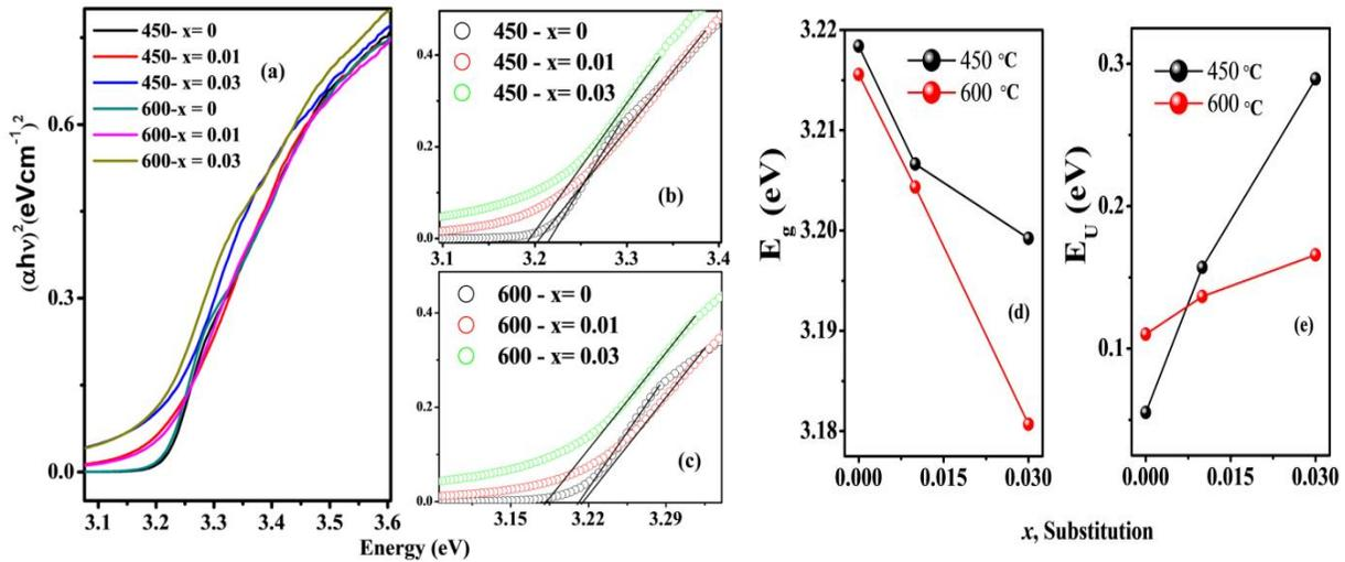
**Figure 3:** Kubelka-Munk plot (a) x=0, 0.01 & x=0.03 at 450 and 600 annealed temperature and (b), (c) Optical energy bandgap estimation using Tauc plot relation respectively (d), (e) bandgap and Urbach energy Vs x, substitution
