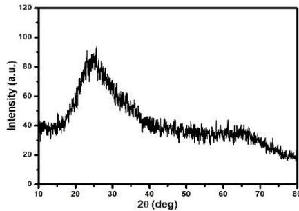
**FIGURE 1.** Typical XRD pattern of holmium doped lithium zinc phosphate glass.
