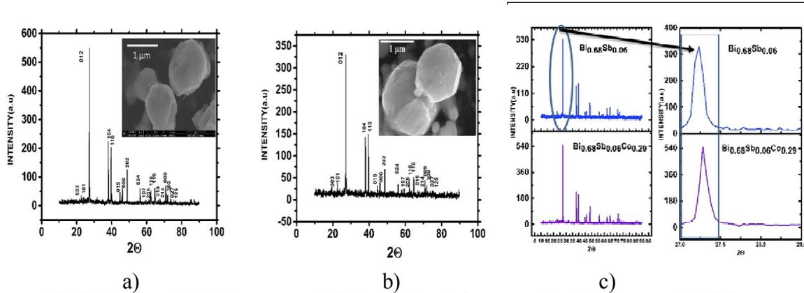
**Figure 1.** FESEM images of (a) XRD pattern and SEM image (inset) of nanocrystalline  $\text{Bi}_{0.94}\text{Sb}_{0.06}$  and (b) XRD pattern and SEM image (inset) of  $\text{Bi}_{0.68}\text{Sb}_{0.06}\text{Co}_{0.29}$  (c) comparison of XRD pattern and main peak shift of  $\text{Bi}_{0.94}\text{Sb}_{0.06}$  and  $\text{Bi}_{0.68}\text{Sb}_{0.06}\text{Co}_{0.29}$
