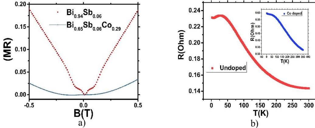
**Figure 2.** a) Magneto resistance MR vs B plot of  $\text{Bi}_{0.94}\text{Sb}_{0.06}$  (red curve) and  $\text{Bi}_{0.68}\text{Sb}_{0.06}\text{Co}_{0.29}$  (blue curve)
