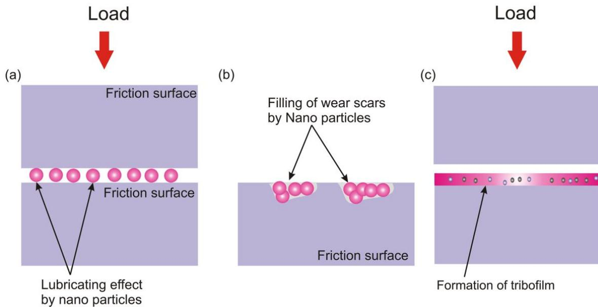
**FIGURE 2.** Schematic presentation of nanoparticles different roles as an additive (a) lubricating effect (b) filling of wear scars (c) formation of tribofilm.
