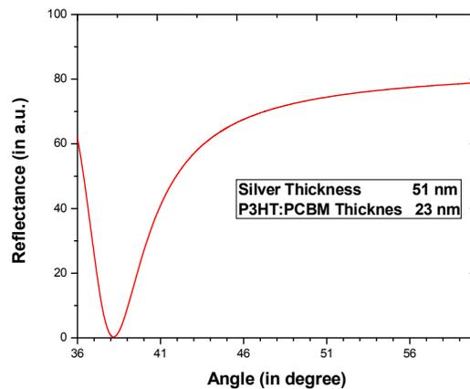
**FIGURE 4.** The reflectance of P3HT-PCBM: Ag film becomes zero at 51 nm thickness of nano Ag film and 23 nm of P3HT-PCBM film.
