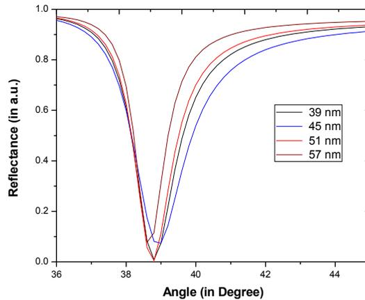
**FIGURE 3.** Dependence of SPR curve on the thickness of metal (silver) film. The parameters used in simulation are Prism BK7 (RI: 1.7225), wavelength – 632.8 nm. The thickness of P3HT:PCBM film is 23 nm.
