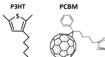
**FIGURE 1:** Chemical structure of PH3T and PCBM
