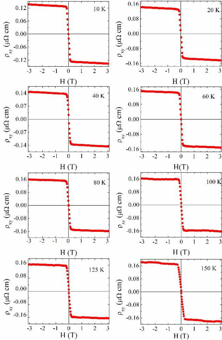
**FIGURE 3:** Isothermal Hall resistivity data of Nickel film measured at various fixed temperatures.
