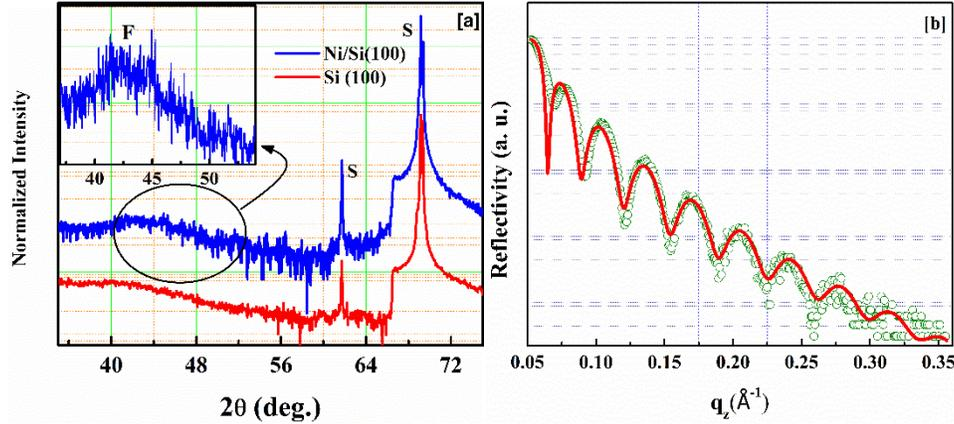
**FIGURE 1:** (a) X-Ray diffraction data of Ni/Si(100) [Blue line]. The Red colored line shows the data for Si (100) substrate. The inset shows the zoomed view indicating the peak corresponding to Ni. (b) X-ray reflectivity of Nickel film. Green open circles show observed data and red line shows the fitted model.
