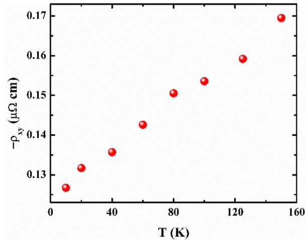
**FIGURE 4:** Temperature dependence of Anomalous Hall resistivity of Nickel film.
