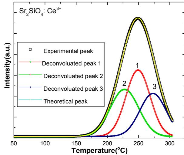
**FIGURE 4.** Deconvoluted glow curve of  $\text{Sr}_2\text{SiO}_4:\text{Ce}^{3+}$  phosphor.
