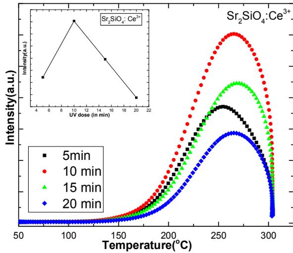
**FIGURE 3.** Thermo-luminescence (TL) glow curve, (inset- UV exposure time vs intensity) of  $\text{Sr}_2\text{SiO}_4:\text{Ce}^{3+}$  phosphor sample.
