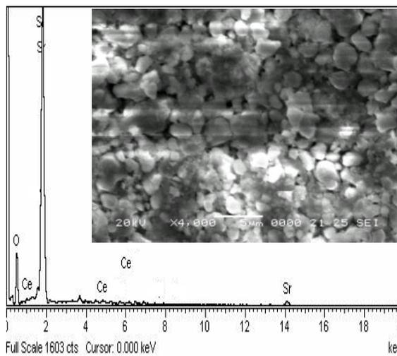
FIGURE 2. EDAX and SEM (inset) of  $\text{Sr}_2\text{SiO}_4:\text{Ce}^{3+}$  phosphor.
