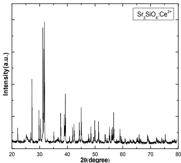
FIGURE 1. XRD pattern of  $\text{Sr}_2\text{SiO}_4:\text{Ce}^{3+}$  phosphor.
