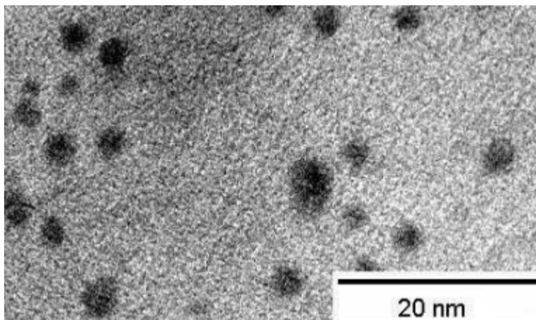
FIGURE 3 SEM image of *in-situ* Ag nano particles
