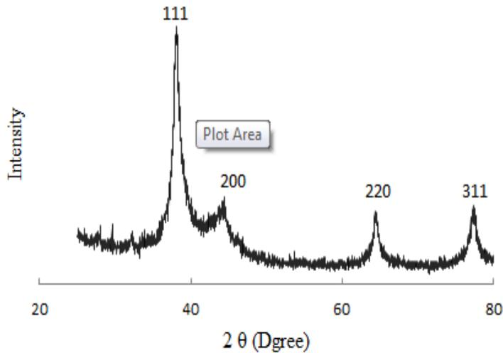
FIGURE 2. X-ray diffraction pattern of Ag nano particles
