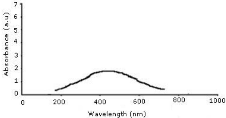
FIGURE 1. The UV/Vis absorption spectra of Ag nano particles
