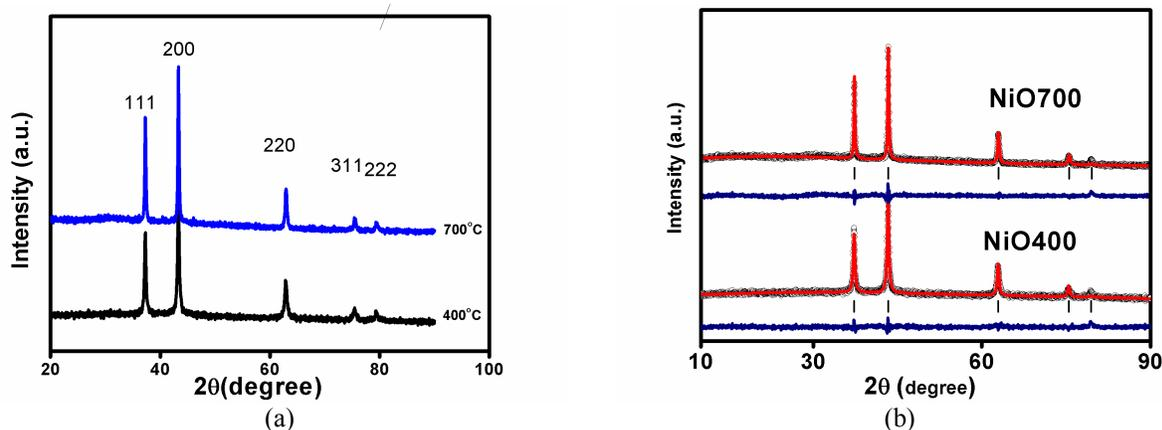
**FIGURE 1.** (a) X ray diffraction pattern of non stoichiometric Ni<sub>1-x</sub>O. (b) Shows the Rietveld refinement fitting of XRD data.
