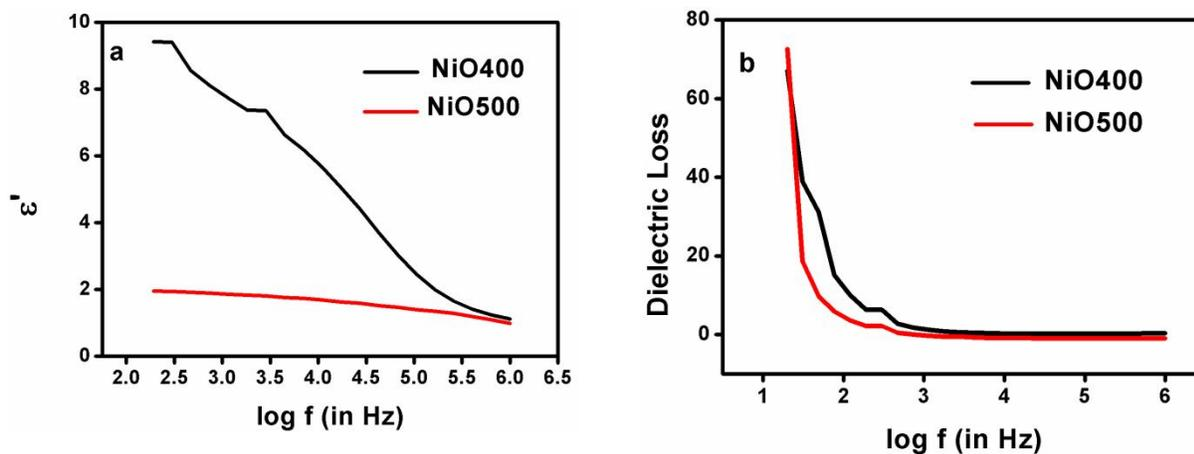
**FIGURE 2.** (a and b) Shows frequency dependent dielectric constant ( $\epsilon'$ ) and loss tangent ( $\tan \delta$ ) of NiO400 and NiO700 samples recorded at room temperature.
