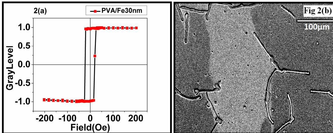
FIGURE 2.2 (a) Magnetization behavior of PVA/Fe30nm as recorded using MOKE 2(b) domain evolution along the easy magnetization axes i.e., 0
