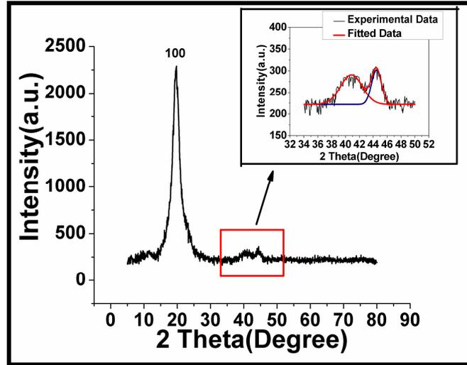
FIGURE 1. GIXRD pattern of Fe deposited on PVA where  $t_{Fe} = 30$  nm. The inset shows close look at Fe peak and smaller PVA peak
