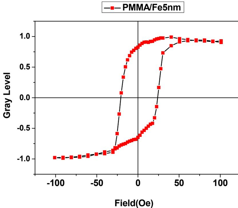
Figure 2: L-MOKE plot of PMMA/Fe films.
