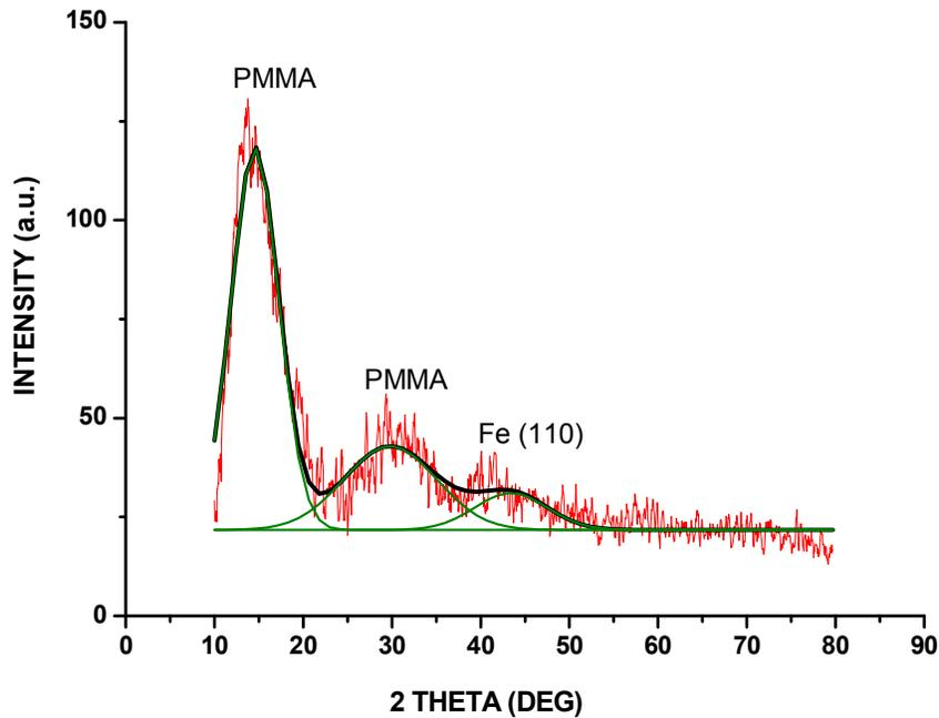
Figure 1: GIXRD pattern of as-deposited PMMA/Fe film.
