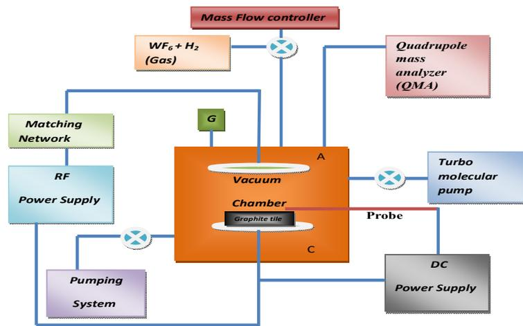
Figure 1 – Block diagram of coating reactor and associated accessories at SVITS.
