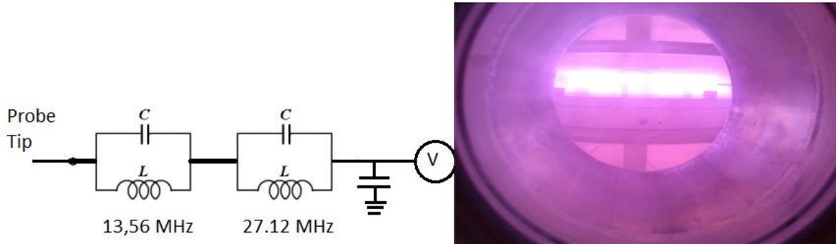
Figure 3. Schematic circuit design of RF compensated Langmuir probe for 13.56MHz and its second harmonic and produced Argon RF plasma in SVITS coating reactor.
