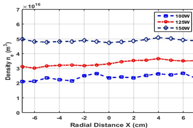
Figure 4 Radial density profile measured at different RF power 3cm above the bottom electrode.
