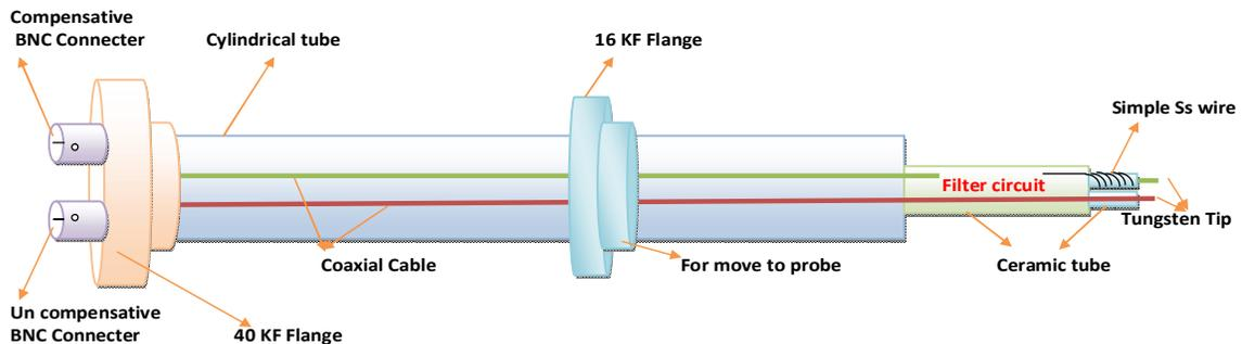
Figure 2 - Schematic of the Langmuir probe used in the system.
