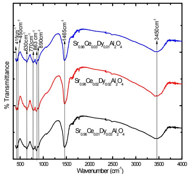
**FIGURE 2.** FTIR spectra of  $\text{Sr}_{1-x}\text{Dy}_{x-z}\text{Ce}_z\text{Al}_2\text{O}_4$  [ $x=0.03, 0.02, 0.01$  and  $z = 0.01, 0.02$  and  $0.03$ ]
