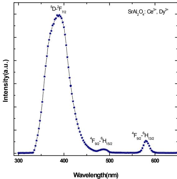
FIGURE 3. PL spectrum of  $\text{Sr}_{0.96}\text{Dy}_{0.03}\text{Ce}_{0.01}\text{Al}_2\text{O}_4$  phosphor
