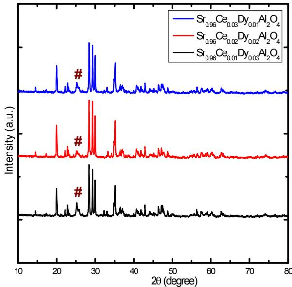
**FIGURE 1.** XRD spectra of  $\text{Sr}_{1-x}\text{Dy}_{x-z}\text{Ce}_z\text{Al}_2\text{O}_4$  [ $x=0.03, 0.02, 0.01$  and  $z = 0.01, 0.02$  and  $0.03$  resp.] phosphors
