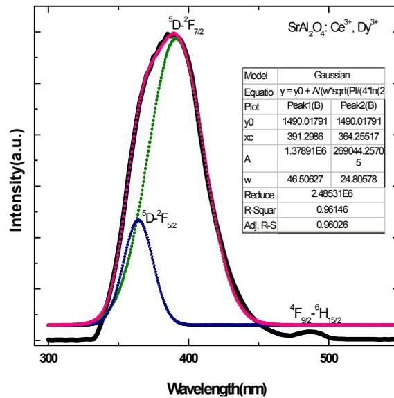
FIGURE 4. Convolved PL spectrum of  $\text{Sr}_{0.96}\text{Dy}_{0.03}\text{Ce}_{0.01}\text{Al}_2\text{O}_4$  phosphor.
