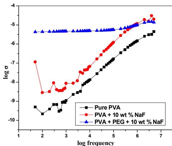
**FIGURE 5.** Variation of a. c. conductivity with frequency for pure PVA, PVA-NaF and PVA-PEG-NaF solid polymer blend electrolyte films.
