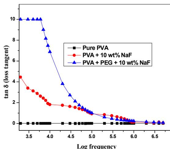
**FIGURE 4.** Variation of dielectric loss tangent ( $\tan \delta$ ) with frequency for pure PVA, PVA-NaF and PVA-PEG NaF solid polymer blend electrolyte films.
