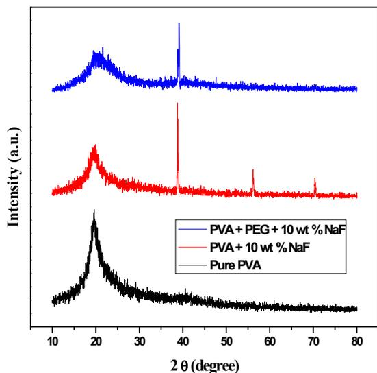
**FIGURE 1.** XRD spectra of pure PVA, PVA-NaF and PVA-PEG-NaF solid polymer blend electrolyte films.
