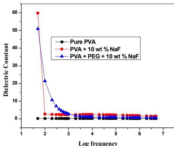
**FIGURE 3.** Variation of  $\epsilon'$  with frequency for pure PVA, PVA-NaF and PVA-PEG-NaF solid polymer blend electrolyte films.
