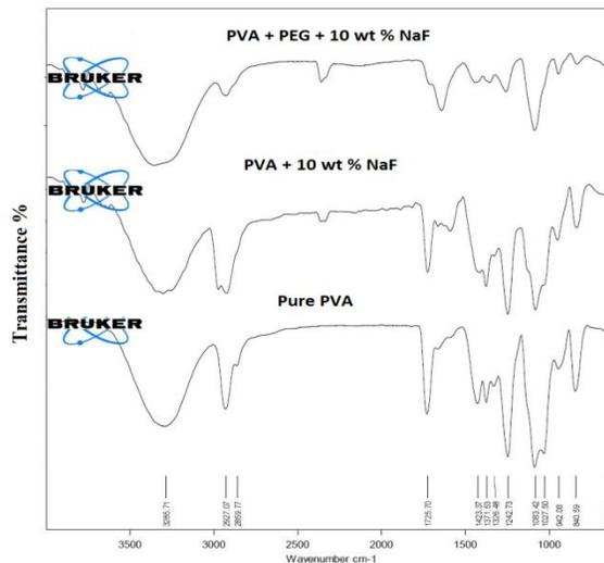
**FIGURE 2.** FTIR Spectra of pure PVA, PVA-NaF and PVA-PEG-NaF solid polymer blend electrolyte films.
