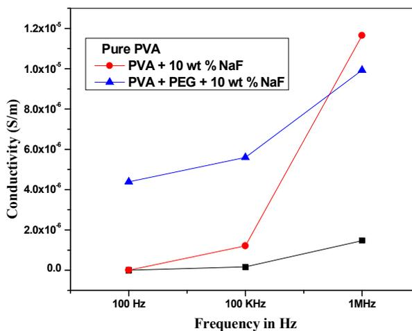
**FIGURE 6.** Variation of a.c. conductivity with different frequency of pure PVA, PVA-NaF and PVA-PEG-NaF solid polymer electrolyte films at different wt %.
