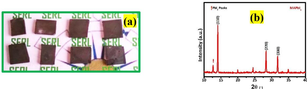
FIGURE 1.(a) Digital images of  $\text{MAPbI}_3$  (b) XRD pattern of the perovskite thin film
