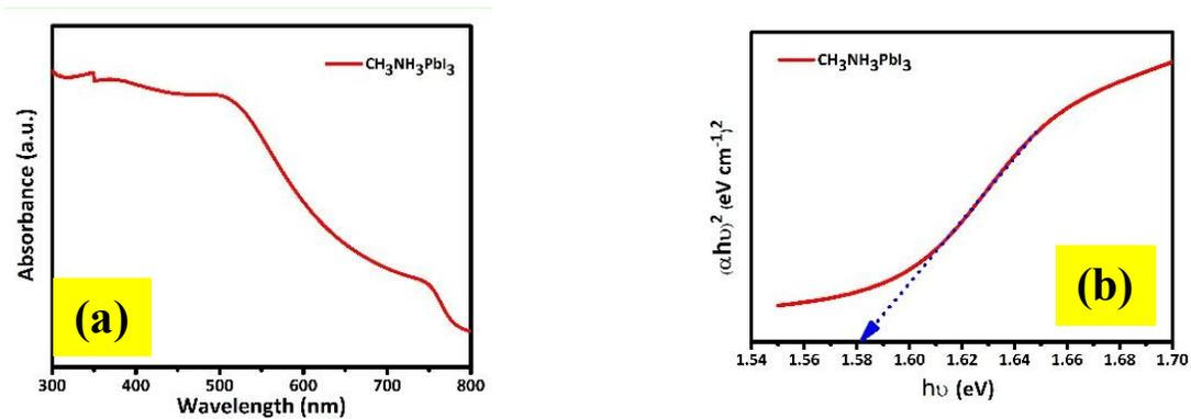
FIGURE 3. (a) Absorbance plot (b) Tauc's plot of the  $\text{CH}_3\text{NH}_3\text{PbI}_3$  thin film
