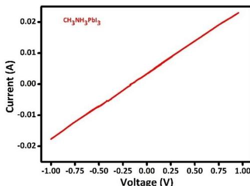
FIGURE 4. I-V characteristics of the CH<sub>3</sub>NH<sub>3</sub>PbI<sub>3</sub> thin film
