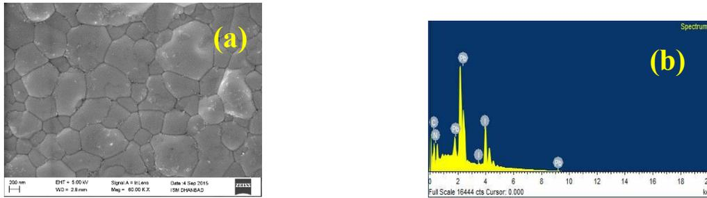
FIGURE 2.(a) Top view FESEM image of  $\text{MAPbI}_3$  thin film (b) EDAX image showing elemental composition
