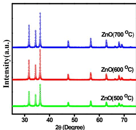
Figure 1. Observed XRD pattern of the ZnO nanoparticles at different temperatures.
