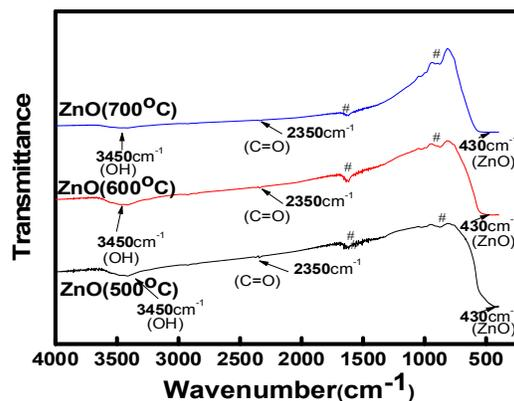
Figure 2. Observed FTIR pattern of the ZnO nanoparticles at different temperatures. (# - residues peaks, probably due to atmospheric moisture and  $\text{CO}_2$  respectively).
